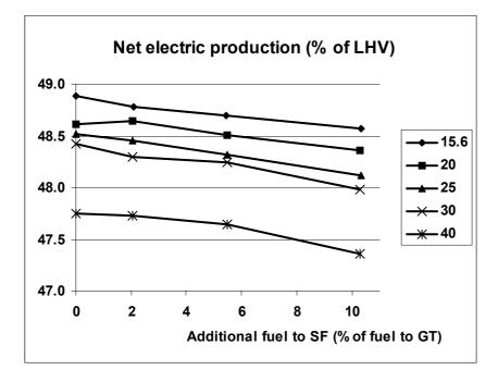
Figure 5 Net electric-power production (in % of the natural gas LHV flow rate) as a function of amount of fuel to supplementary firing (in % of the fuel used in the GT) for five different AC-outlet pressures (bar).
