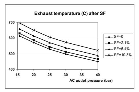
Figure 6 Temperature (°C) in gas-turbine exhaust after supplementary firing, before heat exchange with reformer feed, as a function of AC-outlet pressure (bar) for different amounts of fuel to SF (in % of fuel used for the gas turbine).
