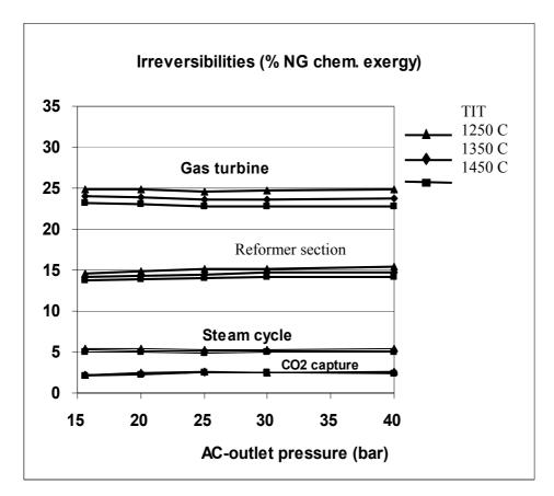
Figure 8 Irreversibilities (in % of NG chemical exergy) for all units in groups for the plant with reforming at three different TITs and various AC-outlet pressures.
