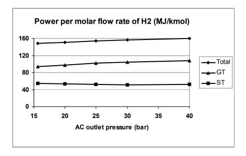
Figure 3 Net mechanical power produced in the total system, by the gas turbine cycle, and by the steam-turbine cycle per flow rate of H2 in the reformed fuel (MJ/kmol  $H_2$ ) as a function of AC-outlet pressure (bar).
