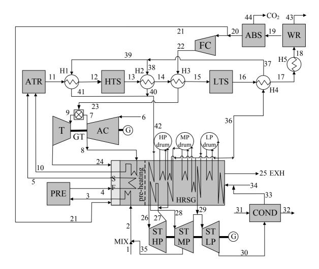
Figure 1 Process flow diagram of the precombustion CO<sub>2</sub>-capture power plant.
