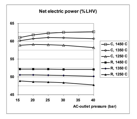
Figure 7 Net electric-power production in percentage of the NG LHV consumption rate as a function of ACoutlet pressure for three different TITs for the conventional plant (C) and the reforming plant (R).
