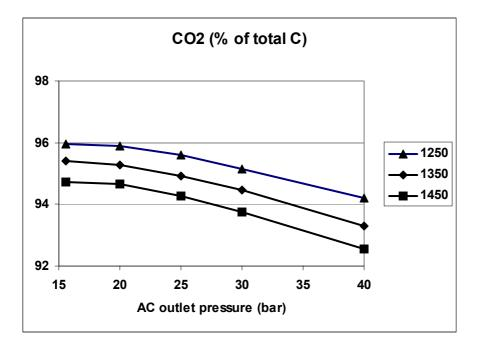
Figure 10 Fraction of all carbon that is present in the form of  $CO_2$  after reforming (stream 17) as a function of AC-outlet pressure for three different TITs.
