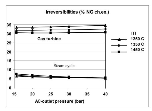
Figure 9 Irreversibilities (in % of NG chemical exergy) for all units in groups for the conventional plant at three different TIT and various AC-outlet pressures.
