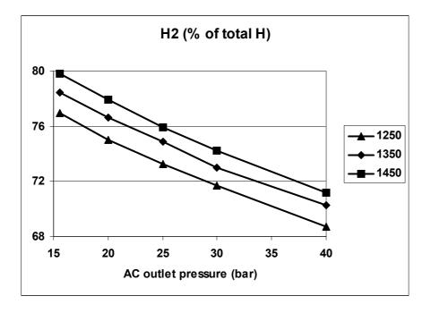
Figure 11 Fraction of all hydrogen that is present in the form of  $H_2$  after reforming (stream 17) as a function of AC-outlet pressure for three different TITs.
