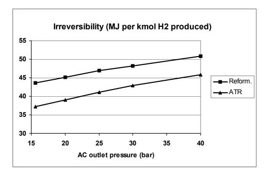
Figure 4 Irreversibility in the ATR and in the entire reformer section, in MJ per kmol H<sub>2</sub> produced as a function of AC-outlet pressure (bar).
